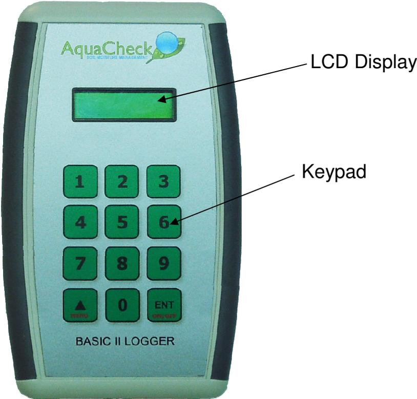
The Scroll(▲)/menu and ENT/ON/OFF pushbuttons have dual functions. The ENT pushbutton turns the logger ON and OFF, whilst during Setup, it functions as an ENTER key. Once the logger is first turned ON, only the function written below the key is operational. All the other keys are inactive.
